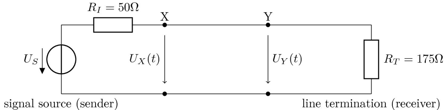
Which voltage value appears at the points X and Y after an infinite amount of time?
